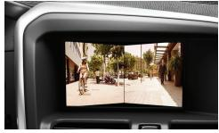
**Front Blind View Camera** Negotiate tight exits with ease, even when visibility is restricted. This camera allows you to "see around corners" with a 180° field of vision in front of the XC60.
