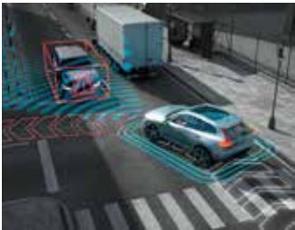
Intersection Braking City Safety includes an intersection braking function that can help to make an accident at a road junction less likely or less harmful. This feature – a world-first when it was introduced in the Volvo XC90 – automatically brakes the car if the driver turns into the path of an oncoming vehicle.
