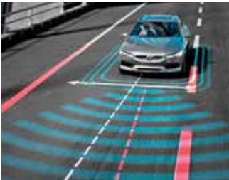
Lane Keeping Aid Fitted as standard, this feature monitors the road ahead and gently steers the car back into its lane if it detects that you're about to cross a lane marking unintentionally. If the car's steering adjustment isn't enough, or if you cross into the other lane, you'll be alerted by gentle vibrations through the steering wheel.
