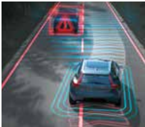
Oncoming Lane Mitigation Using automatic steering assistance, this system helps you avoid collisions with oncoming vehicles. If you drift across the lane markings in the way of an oncoming vehicle, your car steers back.
