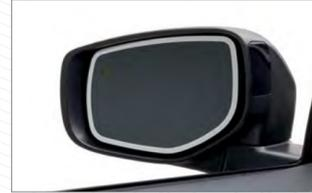
**Auto-Dimming Exterior Mirrors with Approach Light.** Designed to enhance nighttime driving safety by reducing headlight glare. When you approach the vehicle or unlock the doors with the keyless entry system, LED lights in each exterior mirror illuminate the ground next to, and towards the rear of, the vehicle. During nighttime driving, the Auto-Dimming Exterior Mirrors dim in unison with the Auto-Dimming (Interior) Mirror when glare is detected.
