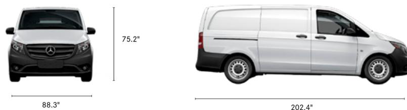
All measurements in inches. All width measurements include mirrors.
