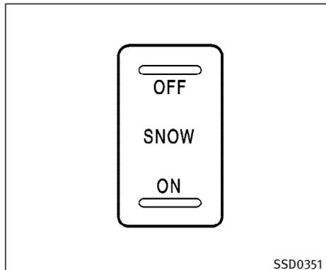
For driving or starting the vehicle on snowy roads or slippery areas, turn on the SNOW mode switch and the indicator light on the switch will illuminate. When the SNOW mode is activated, engine output is controlled to avoid wheel spin.
