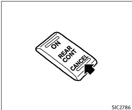
The rear control cancel switch is located on the center console.
