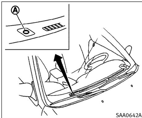
**Be sure not to put anything on top of the photo sensor
