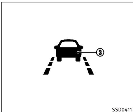
When the vehicle approaches either the left or the right of the traveling lane while driving over approximately 45 MPH (72 km/h), the LDW indicator ③ on the instrument panel flashes and a chime sounds to alert the driver.
