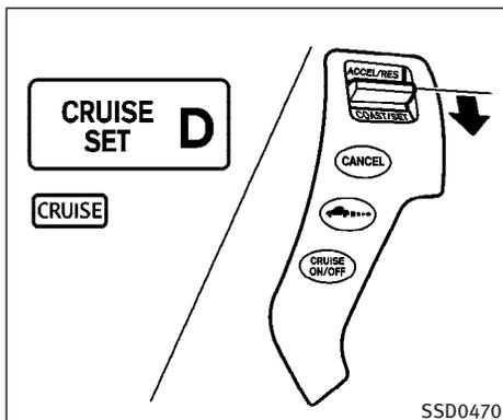
**To set cruising speed**, accelerate your vehicle to the desired speed, push the SET/COAST switch and release it. (The CRUISE SET indicator will come on in the display.) Take your foot off the accelerator pedal. Your vehicle will maintain the set speed.
