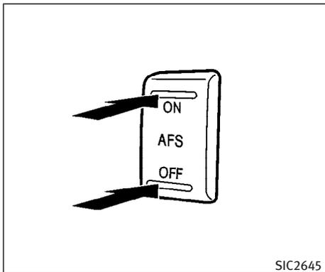
To turn the AFS off, push the OFF side of the AFS OFF switch. (The AFS OFF indicator light will illuminate.) Push the ON side of the switch to turn the system on again.
