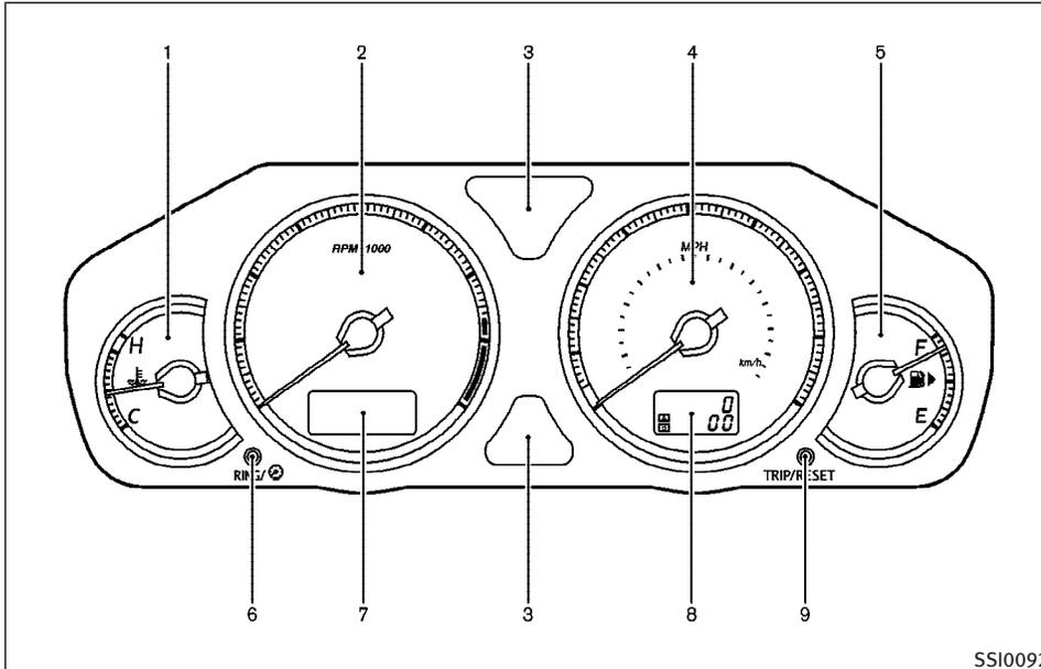
9. TRIP/RESET knob for twin trip odometer (P.2-5)
