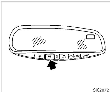
3. Using both hands, simultaneously push and hold both the HomeLink<sup>®</sup> button you want to program and the hand-held transmitter button. DO NOT release the buttons until step 4 has been completed.
