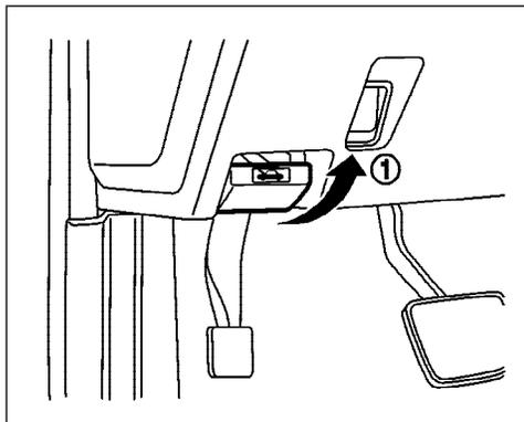
1. Pull the hood lock release handle ① located below the instrument panel; the hood will then spring up slightly.
