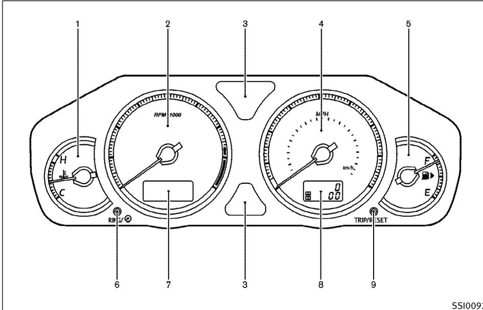
\*: The needle indicators in the speedometer, tachometer, engine coolant temperature gauge and fuel gauge may move slightly after the ignition switch is pushed to the LOCK position. This is not a malfunction.
