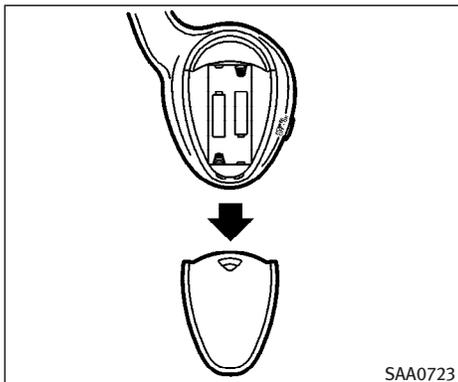
Make sure that the  $\oplus$  and  $\ominus$  ends on the batteries match the markings inside the compartment.
