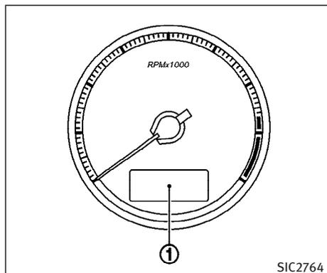
The dot matrix liquid crystal display ① is located under the tachometer to display the automatic transmission position indicator, the Intelligent Cruise Control (ICC) system (if so equipped) information and the Intelligent Key operation information.
