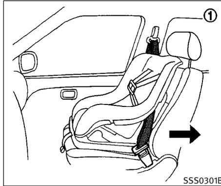
1. Position the child restraint on the front passenger seat. **It should be placed in a front facing direction only.** Move the seat to the rearmost position. Adjust the head restraint to its highest position. Always follow the child restraint manufacturer's instructions. **Child restraints for infants must be used in the rear facing direction and therefore must not be used in the front seat.**
