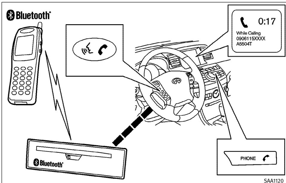
Your INFINITI is equipped with the Bluetooth® Hands-Free Phone system. If you are an owner of a Bluetooth® enabled cellular phone, you can set up the wireless connection between your cellular phone and the in-vehicle phone module. With
