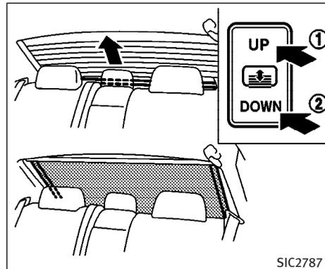
The rear sunshade operates when the ignition switch is in the ON position.
