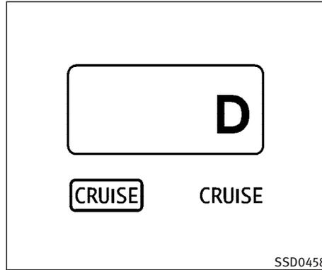
When the ignition switch is pushed to the ON position, the indicators come on as illustrated to check for a burned-out bulb, and it turns off when the engine is started.
