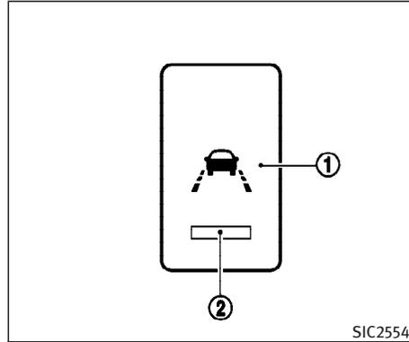
The Lane Departure Warning (LDW) system will blink an indicator light on the instrument panel and sound a chime to alert the driver if the vehicle is traveling close to either the left or the right of a traveling lane with detectable lane markers.
