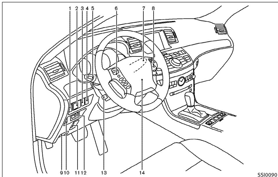
1. Instrument brightness control switch (P.2-30)
