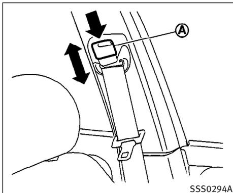
To adjust, push the button (A), and then move the shoulder belt anchor to the desired position, so that the belt passes over the center of the shoulder. The belt should be away from your face and neck, but not falling off of your shoulder. Release the button to lock the shoulder belt anchor into position.
