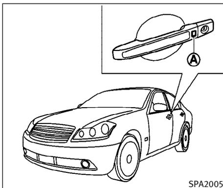
When you carry the Intelligent Key with you, you can lock or unlock all doors by pushing the door handle request switch (A) within the range of operation.
