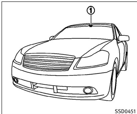
The Lane Departure Warning (LDW) system warns the driver when the vehicle is traveling close to either the left or the right of a traveling lane with detectable lane markers. It operates at approximately 45 MPH (72 km/h) and above. The system monitors lane markers of the traveling lane using the camera unit ① located inside the map light cover.
