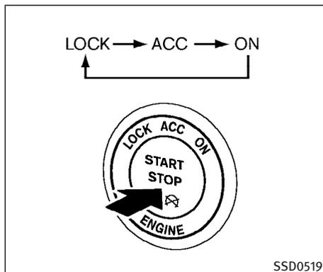
When the ignition switch is pushed without depressing the brake pedal, the ignition switch position will illuminate as follows:
