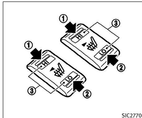
The rear outboard seats are warmed by built-in heaters. The switches, located on the inside of the rear center armrest, can be operated independently of each other.
