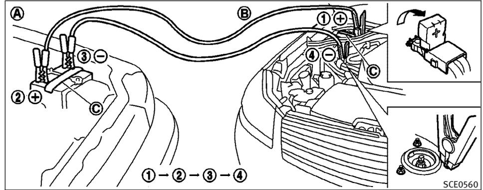
2. If the booster battery is in another vehicle (A), position the two vehicles (A and B) to bring their batteries into close proximity to each other.
