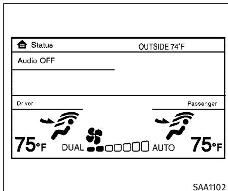
You can individually set driver and front passenger side temperature and air flow using each temperature control button and manual air flow control button.
