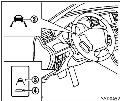
The LDW system can be turned on or off by pushing the LDW switch ③. When the system is on, the LDW system ON indicator ④ illuminates.
