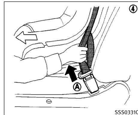
4. Allow the seat belt to retract. Pull up **(A)** on the shoulder belt to remove any slack in the belt.
