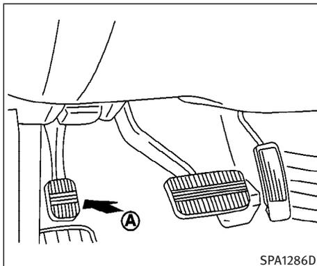
**To apply:** Fully depress the parking brake pedal (A).
