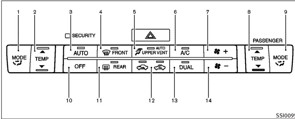
1. "MODE" manual air flow control button (driver side)
