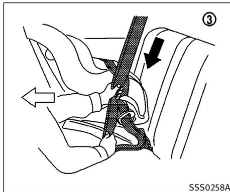
3. Pull on the shoulder belt until all of the belt is fully extended. At this time, the seat belt retractor is in the automatic locking mode (child restraint mode). It reverts back to emergency locking mode when the belt is fully retracted.
