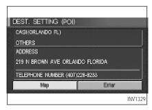
When the Info key next to the facility name of your choice is selected in step 2, the display shows the detailed [Address] and [Telephone number] of the selected facility, and the Map and Enter keys.
