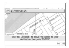
6. If necessary, operate the joystick to adjust the location of the destination (waypoints). Press the ENTER button. Select the Destination key to confirm. The [DEST. SETTING] screen will be displayed. To set the destination (waypoints), refer to "Making the system guide the route with detailed options" on page 5-27.
