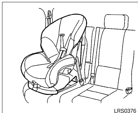
Front facing (outboard) — step 1
