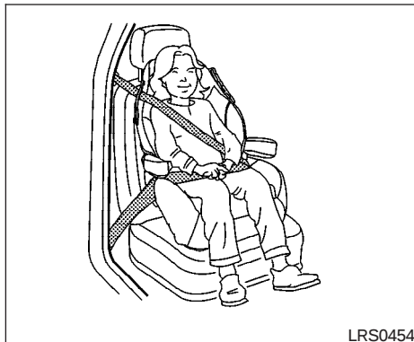
Booster seat installation on front passenger seat
