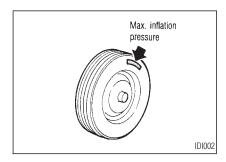
Do not exceed the maximum inflation pressures shown on the side wall of the tire.
