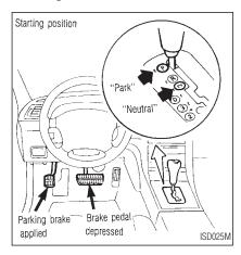
After starting the engine, fully depress the foot brake pedal and push the selector lever button before shifting the selector lever from "P" to the "D", "R", "3", "2" or "1" position. Be sure the vehicle is fully stopped before attempting to shift the selector lever from or to "P" or "R".
