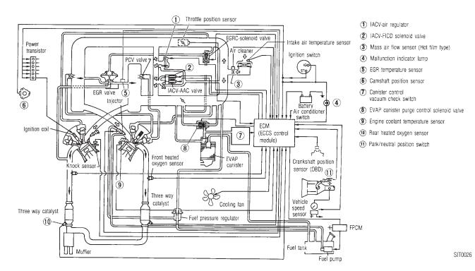
To get the most from an engine—in the way of performance, smooth driveability, economy and control of harmful emissions—a number of decisive factors must be controlled as precisely as possible under all driving conditions. These "factors" include the following:
