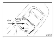
To fully open the driver side window, completely press down the switch and release it; it need not be held. The window will automatically open all the way. To stop the window, just pull up the switch toward the "CLOSE" side.
