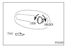
To lock the door, turn the key toward the front of the vehicle.
