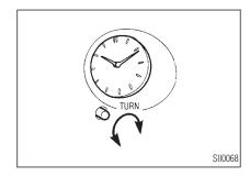
The time can be adjusted by turning the knob.
