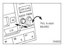
Push then pull the BAL (BALANCE) control knob to adjust the volume between the right and left speakers.
