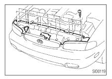
Before adjusting the headlights, make sure that all of the tires are properly inflated, the vehicle is on level ground and there is no excess weight in the vehicle that would effect the level of the vehicle.
