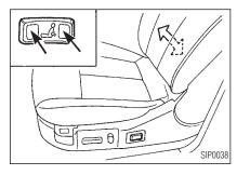
Push either side of the switch to adjust the seat lumbar area.
