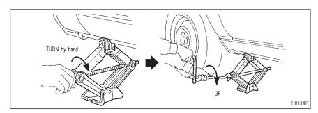
1. Place the jack directly under the jack-up point as illustrated above so that top of the iack contacts the vehicle at the jack up point. Align the center of both the jack head and the notch at the jack up point as shown. Also fit the notched portion of the vehicle in the groove of the jack head as shown.
