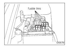
If any electrical equipment does not operate and fuses are in good condition, check the fusible links. If any of these fusible links are melted, replace only with genuine parts. See your INFINITI dealer.
