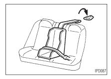
If your child restraint has a top strap, install the anchor bracket to the provided anchor point. Anchor bracket hardware must be installed. The top strap anchor bracket hardware is available through your INFINITI dealer.
