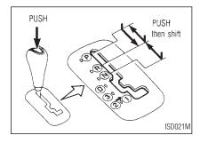
Push the button to shift into "P", or from "N" to "R" and "P" to "R". All other positions can be selected without pushing the button.
