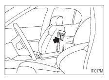
The cold tire pressure is shown on the tire placard affixed to the center console lid.
