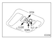
To open the roof, keep pressing the switch to the "OPEN" side.
