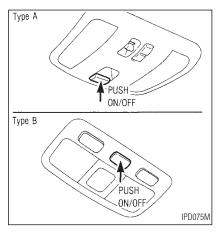
With the console light switch turned on, the light will come on by turning the headlight and turn signal switch to the "<code>EDGE</code>" or "<code>DOSTION</code> or position. The light is designed to illuminate the switches, etc. on the center console and the automatic transmission shift
