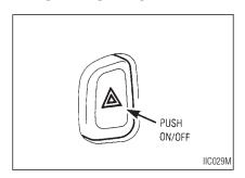
Push the switch on to warn other drivers when you must stop or park under emergency conditions. All turn signal lights will flash.
