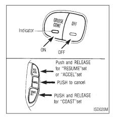
**To turn on the cruise control,** push the main switch on. The indicator light on the switch will come on.
