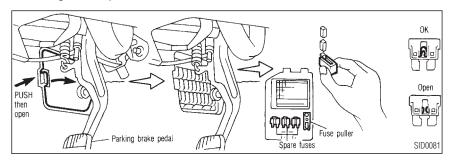
If any electrical equipment does not operate, check for an open fuse.
