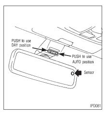
The inside mirror is designed so that it automatically changes reflection according to the intensity of the headlight of the following vehicle.
