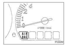
The supplemental air bag light, displaying "AIR BAG" in the instrument panel, monitors the circuits of the supplemental air bag. The circuits monitored by the supplemental air bag light are the diagnosis sensor unit, supplemental air bag modules and all related wiring.
