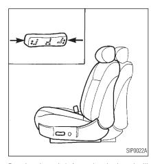
Pressing the switch forward or backward will slide the seat forward or backward to the desired position.
