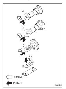
All other lights are either type A, B or C. When replacing a bulb, first remove the lens and/or
