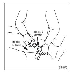
1. Insert the tongue into the buckle marked
