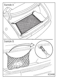
Do not put heavy objects in the cargo net. The net is designed only to hold light packages or objects in place while driving.
