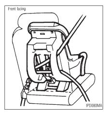
2. Route the seat belt tongue through the child restraint and insert it into the buckle until you hear and feel the latch engage.
