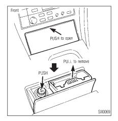
The cigarette lighter operates when the ignition switch is in the "ACC" or "ON" position.
