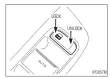
Operating the lock-unlock switch will lock or unlock all doors.
