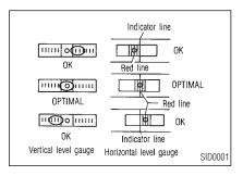
The horizontal gauge adjustment screw is above the headlight. The inner red line should align with the "O" mark on the indicator.
