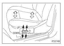
Pull or lower either side of the switch to adjust the seat cushion to the desired angle and height.
