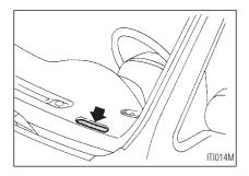
The vehicle identification number plate is attached as shown. This number is the identification for your vehicle and is used in the vehicle registration.
