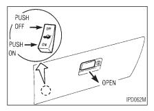
When the cancel switch located inside the glove box is "OFF", the trunk lid cannot be opened with the trunk lid release switch or the remote controller. It can be opened only with the master key or wallet key.
