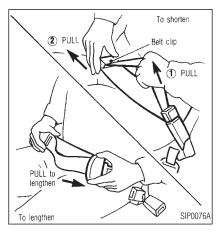
2. To lengthen, hold the tongue at a right angle to the belt and pull on the belt.
