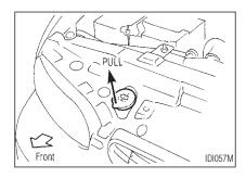
Add fluid when the low washer fluid warning light comes on. Add a washer solvent to the water for better cleaning. In the winter season, add a windshield washer anti-freeze. Follow the manufacturer's instructions for the mixture ratio.
