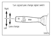
Move the lever up or down to signal the turning direction. When the turn is completed, the turn signals cancel automatically.
