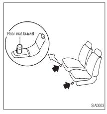
Your INFINITI model includes floor mat brackets to act as floor mat positioning aids. Position the mat and place the floor mat bracket hook through the floor mat grommet hole. Repeat this procedure for both the driver side and front passenger side floor mats.
