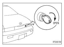
To open the trunk lid, turn the key clockwise. To close, lower and push the trunk lid down securely.
