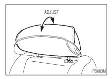
To adjust the head restraint, push it forward or rearward as shown.
