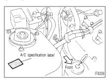
The air conditioner specification label is affixed on the strut tower as shown.
