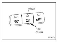
To defog the rear window glass and the outside door mirrors, start the engine and push the switch on. (The indicator light will come on.) Push the switch again to turn the defogger off.
