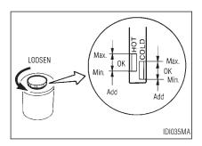
The fluid level should be checked using the "HOT" range on the dipstick at fluid temperature of 122 to 176°F (50 to 80°C) or using the "COLD" range on the dipstick at fluid temperature of 32 to 86°F (0 to 30°C).
