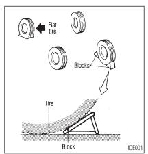
Place suitable blocks at both the front and back of the wheel diagonally opposite the flat tire to prevent the vehicle from rolling when it is jacked up.
