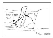
To open, push the cup holder opener switch. To close, lower the cup holder lid and push down lightly.
