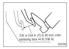
From the released position, depress the parking brake pedal slowly and firmly, and check the distance between the initial and final position of the pedal. If it is out of the range shown above, see your INFINITI dealer.
