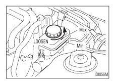
Check the fluid level in the reservoir. If the fluid is below the Min. line or the brake warning light comes on, add DOT 3 fluid up to the Max. line. If fluid must be added frequently, the system should be checked by your INFINITI dealer.
