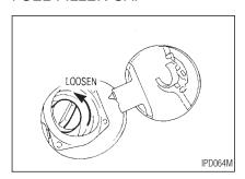
The fuel filler cap is a screw-on ratcheting type. Tighten the cap clockwise until ratcheting clicks are heard.
