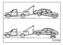
If you have to tow an automatic transmission model with four wheels on ground or with front wheels raised (with rear wheels on ground)
