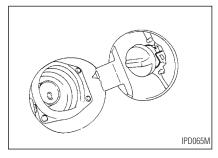
Put the fuel filler cap on the cap holder while refueling.
