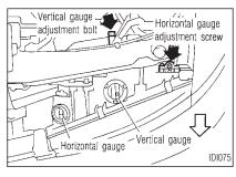
You will see two gauges on the headlight. The gauge on the side further away from the engine is the vertical gauge. The gauge that is closer to the engine is the horizontal gauge.
