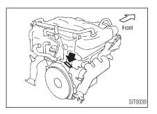
The number is stamped on the engine as shown.
