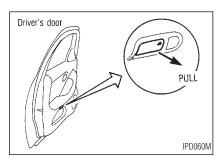
To open the trunk lid, pull the release switch. To close, push the trunk lid down securely.
