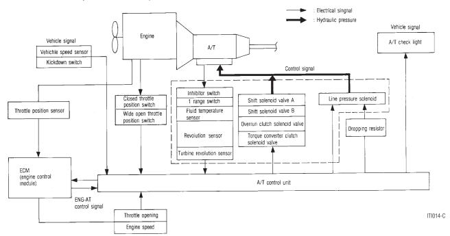
The function of an automotive transmission, is to provide a means of matching engine speed and vehicle speed in such a way that the engine is kept in the most efficient RPM range at all times.
