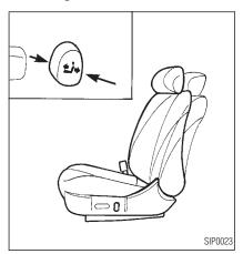
Moving the recline switch forward or backward will move the seatback forward or backward to the desired position.
