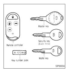
The master key and wallet key can be used for all the locks. The security key cannot be used for the trunk lid or glove box locks. To protect belongings when you leave a key with someone, give them the security key only. Never leave this key in the vehicle.
