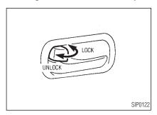
To lock from the outside without a key, move the inside lock knob to the "LOCK" position. Then close the door
