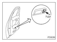
To open the fuel filler lid, push the opener switch. To lock, close the fuel filler lid securely.
