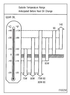
For differential gear oil, 80W-90 is preferable for ambient temperatures below 104°F (40°C).
