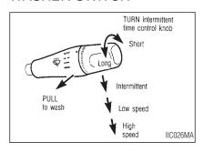
The windshield wiper and washer operates when the ignition key is in the "ACC" or "ON" position.
