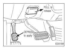
**To apply:** Fully depress the parking brake pedal.
