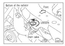
2. Open the radiator cap and drain valve.
