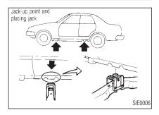
Jacking up and removing wheel
