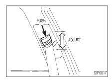
To adjust, push the release button, and then move it to the desired position, so that the belt passes over the center of the shoulder. The belt should be away from your face and neck, but not falling off of your shoulder.
