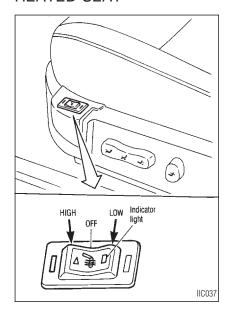
The front seats are warmed by built-in heaters. The switches located on the side part of the seats can be operated independently of each other.
