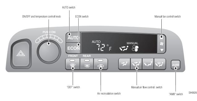
Start the engine and operate the controls to activate the air conditioner.
