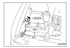
Check the coolant level in the reservoir tank when the engine is cold. If the coolant level is below "MIN", add coolant up to the "MAX" level. If the reservoir tank is empty, check the coolant level in the radiator **when the engine is cold.** If there is insufficient coolant in the radiator, fill the radiator with coolant up to the filler opening and also add it to the reservoir tank up to the "MAX" level.
