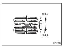
Open or close, and adjust the air flow direction of ventilators.
