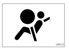
The supplemental air bag warning light, displaying in the instrument panel, monitors the circuits of the supplemental front air bag, supplemental side air bag and curtain side-impact air bag systems, and pretensioner seat belt. The circuits monitored by the air bag warning light are the diagnosis sensor unit, satellite sensors, front air bag modules, side air bag modules, curtain side-impact air bag modules, and all related wiring,
