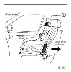
Position the child restraint on the front passenger seat. It should be placed in a front facing direction only. Move the seat to the rear most position. Adjust the head restraint to its highest position. Always follow the child restraint manufacturer's instructions. Child restraints for infants must be used in the rear facing direction and therefore must not be used in the front seat.
