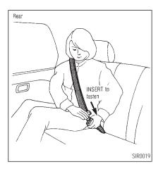
Slowly pull the seat belt out of the retractor and insert the tongue into the buckle until it snaps.
