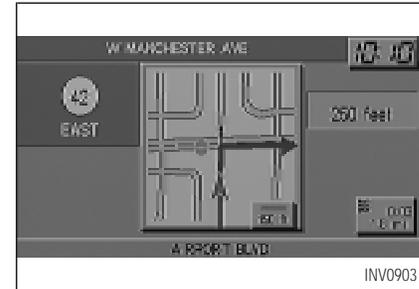
Route guidance is executed using voice and screen instruction. When the vehicle approaches an intersection where you need to turn, the voice guidance tells you the direction to take.
