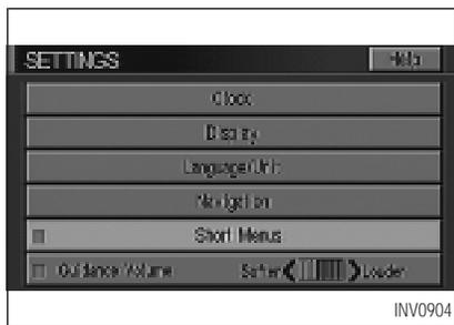
To make the Infiniti Navigation System easier to use, there is a short menu function in which various operation items are reduced in number. When the indicator is illuminated, the short menus (Easy Mode) are displayed. When the indicator is turned off, the default naviga-
