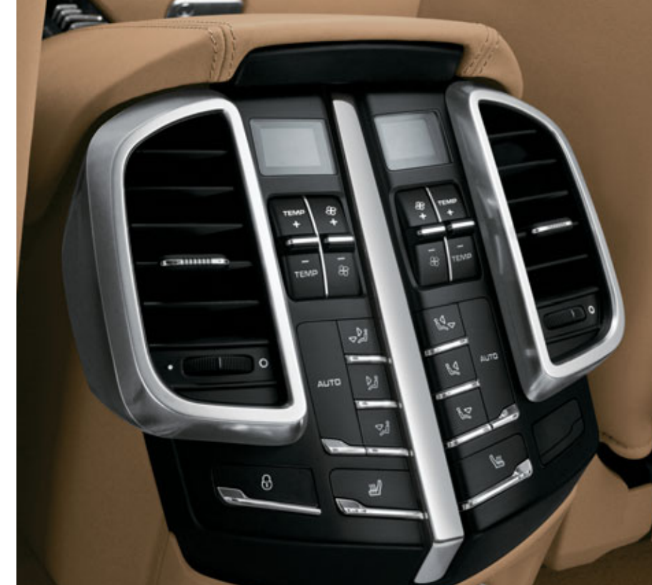
Four-zone climate control for rear seat area
