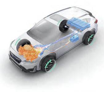
In **everyday driving**, the system will run on a combination of electric and gas power. It can also recover energy via regenerative braking.
