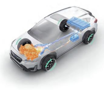
In everyday driving, the system will run on a combination of electric and gas power. It can also recover energy via regenerative braking.
