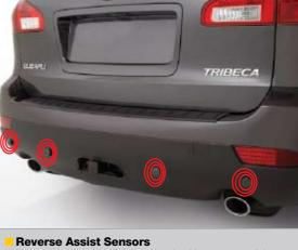
Helps provide added confidence when backing up or parallel parking. When reversing, audible warnings alert the driver as the vehicle approaches large objects in its path. The intermittent tone increases in frequency as the vehicle gets closer to the object. H481SXA100
