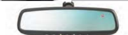
Auto-Dimming Mirror with Compass and HomeLink* Mirror automatically dims when headlights are detected from behind the vehicle. Features an electronic compass with a non-reflective display. Three integrated HomeLink buttons can be programmed to operate roof-rack door openers and other HomeLink devices. H01SA070
