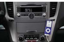
Media Hub Play music through the vehicle's stereo system from your iPod or USB music storage device and control it using the radio and steering wheel buttons. Displays song information on radio screen and charges most portable music devices. H011SA000 (Excludes NAV)
