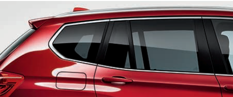
Privacy glass in the rear cabin windows helps suppress excessive heating of the interior and also filters the sun's harmful UV rays more effectively than clear glass.
