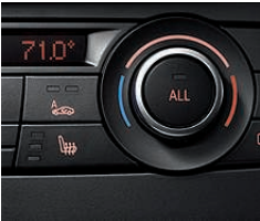
Heated front seats (shown) and heated rear seats are a welcome feature for driver and front passenger in cooler weather. By pressing the icon button, seat surface and backrest are heated and quickly radiate comfortable warmth in your choice of settings.
