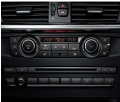
Automatic climate control system allows occupants to select a specific cabin temperature and choice of fan speeds, as well as automatic or manual airflow and recirculation. The automatic recirculation control activates whenever certain air pollutants are detected. The system also includes defrost/demist and MAX A/C functions.
