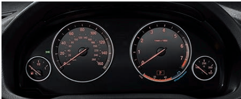
Instrument panel features a red backlit speedometer and tachometer. Centered between the two easy-to-read analog instruments is the on-board computer with liquid crystal display providing additional important driving information.
