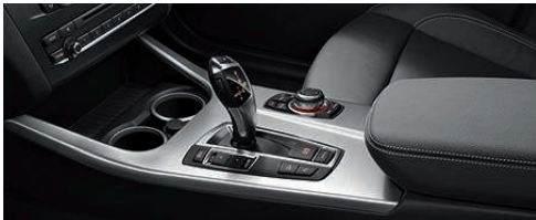
8-speed STEPTRONIC automatic transmission with Adaptive Transmission Control (ATC) provides extremely fast synchronized shifting in either the Sport or Manual shift mode. By increasing the number of gears to eight, the transmission provides a more efficient shifting sequence and improved fuel economy. 8-speed Sport Automatic transmission (not shown) includes Adaptive Transmission Control (ATC) with Sport or Manual shift modes and steering wheel-mounted paddle shifters. When in Sport mode, shifts can be generated via the console-mounted shift lever or the paddle shifters.
