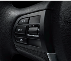
Dynamic Cruise Control lets you set and keep to a chosen speed above 20 mph, including automatic application of the brakes when driving downhill. It is activated and regulated via controls positioned on the left side of the steering wheel, and deactivated by applying the brakes or switching off the feature. 2
