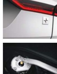
The front suspension is further stabilized by a Polestar Engineered strut bar. This contributes to even more precise, responsive steering characteristics at all speeds and more controlled handling through the curves.
