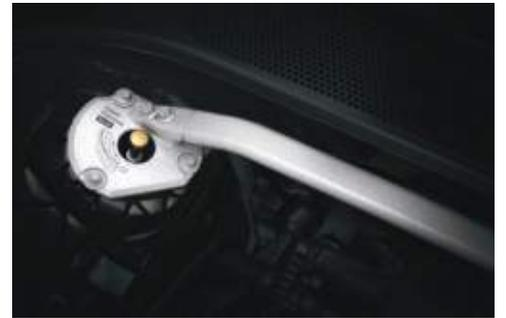
The front suspension is further stabilized by a Polestar Engineered strut bar. This contributes to even more precise, responsive steering characteristics at all speeds and more controlled handling through the curves.
