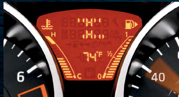
AWD Display – A digital readout between the gauges provides real-time AWD feedback for all four corners.
