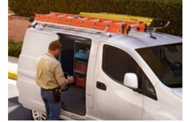
Integrated roof rack-mounting points help secure racks and reduce likelihood of rusting caused by drilling into sheet metal. 1
