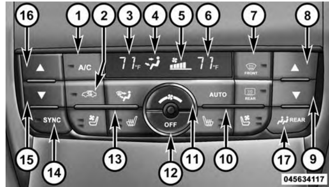
Automatic Temperature Control (ATC) Panel
