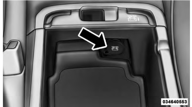
Front Center Console Outlet
