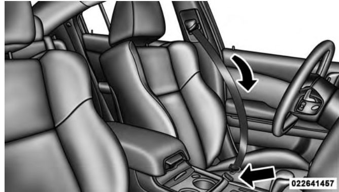
Pulling Out The Latch Plate
