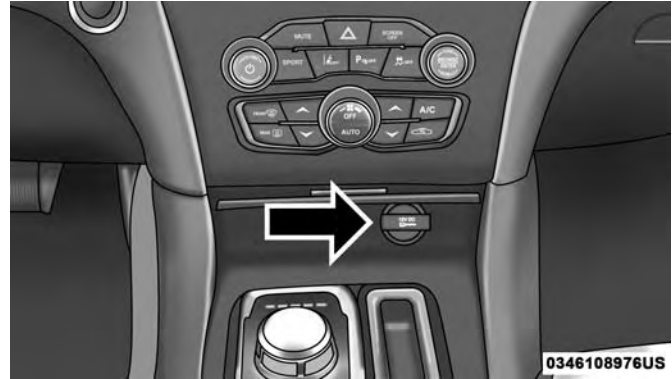
Front Power Outlet
