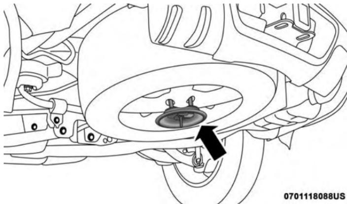
**Road Wheel Installed In Spare Location**
