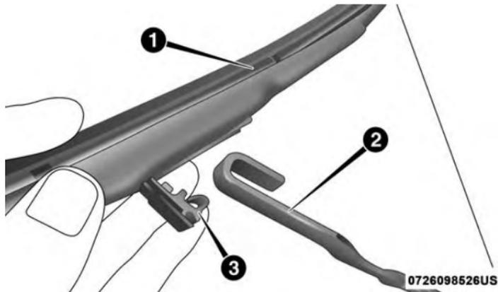
Wiper Blade Removed From Wiper Arm
