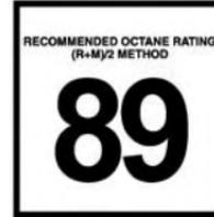
This engine is designed to meet all emissions regulations and provide satisfactory fuel economy and performance when using high-quality unleaded gasoline having an octane range of 87 to 89 as specified by the (R+M)/2 method. The use of 89 octane "Plus" gasoline is recommended for optimum performance and fuel economy.
