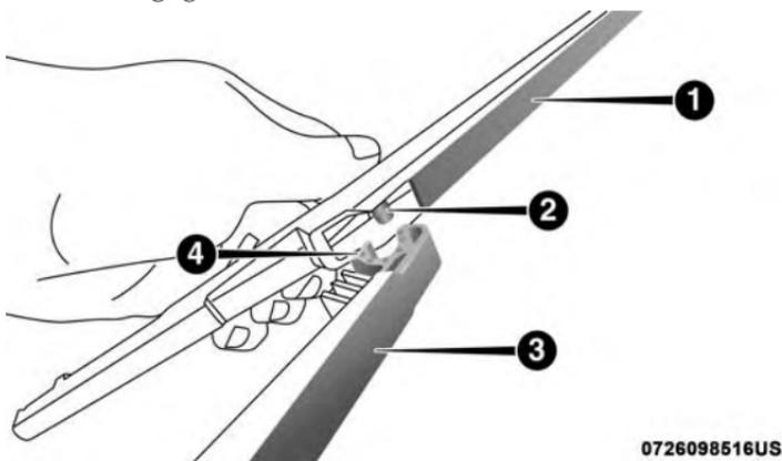
Wiper Blade Removed From Wiper Arm
