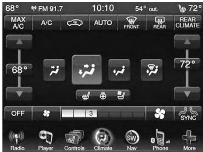
Uconnect 3/3 NAV Automatic Tri-Zone Temperature Controls
