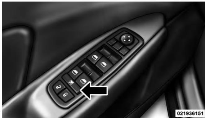
Window Lockout Switch
