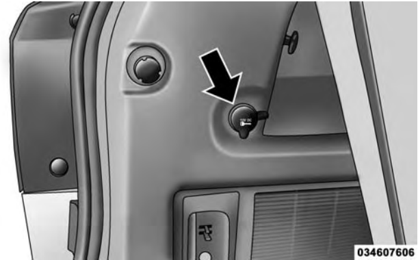
Rear Cargo Area Power Outlet
