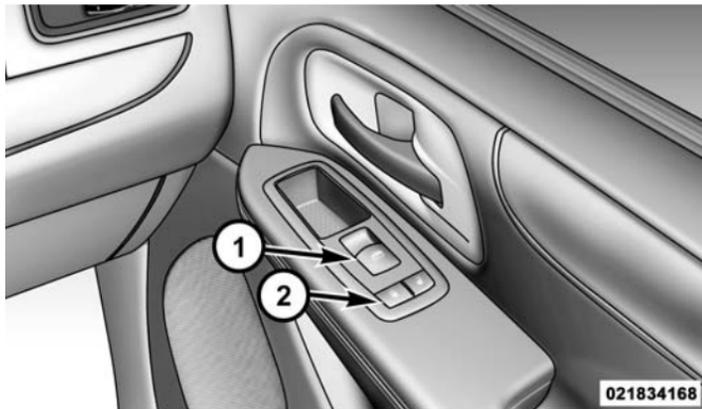
**Front Passenger Power Window And Door Switches**
