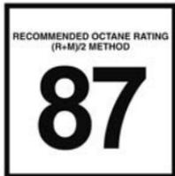
This engine is designed to meet all emissions regulations and provide optimum fuel economy and performance when using high quality unleaded "Regular" gasoline having a posted octane number of 87 as specified by the (R+M)/2
