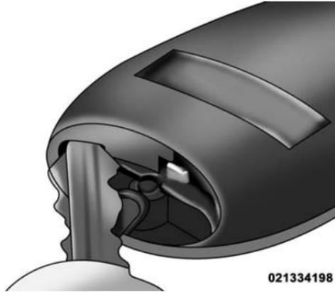
Inserting Key Into Key Fob Case Slot
