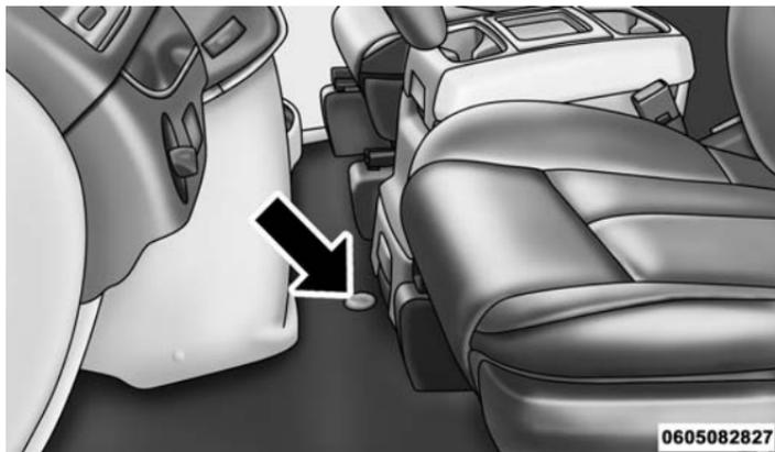
Winch Cover Assembly Plug (If Equipped)
