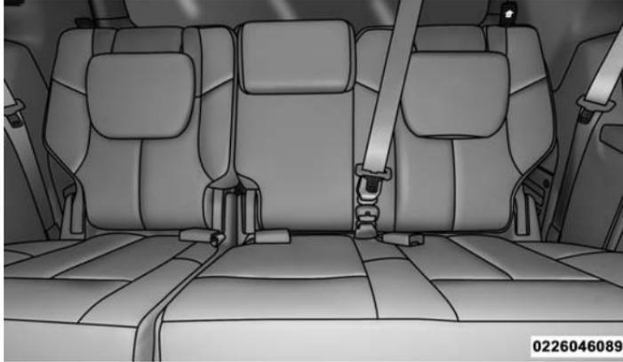
**Mini-Latch And Buckle Connected**
