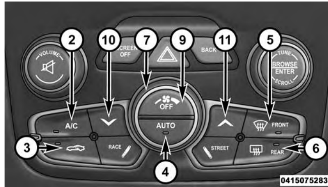
Automatic Climate Controls
