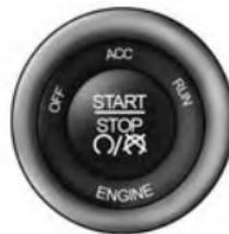
This feature allows the driver to operate the ignition switch with the push of a button, as long as the ENGINE START/STOP button is installed and the Remote Start/Keyless Enter-N-Go Key Fob is in the passenger compartment.
