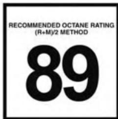
This engine is designed to meet all emissions regulations and provide satisfactory fuel economy and performance when using high quality unleaded gasoline having a posted octane number range of 87 to 89 as specified by the (R+M)/2 method. The use of 89 octane "Plus" gasoline is recommended for optimum performance and fuel economy.
