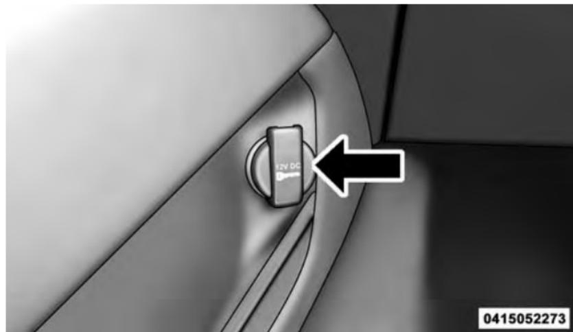
**Power Outlet — Integrated Center Stack Front**
