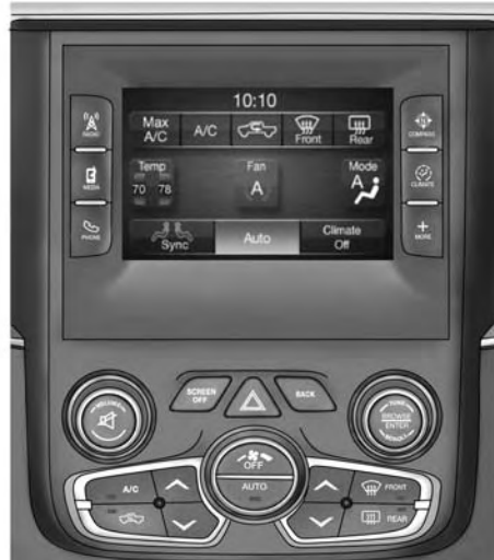
5.0 With Automatic Temperature Controls
