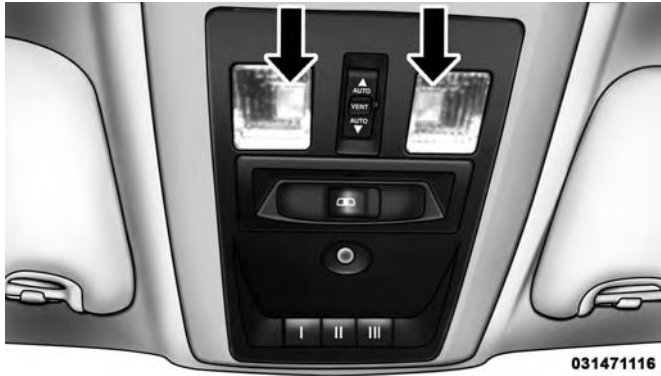
Front Courtesy/Reading Lights
