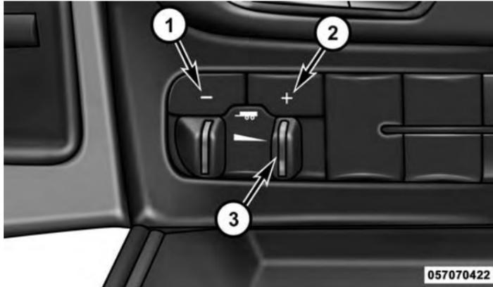
**Integrated Trailer Brake Module (ITBM)**
