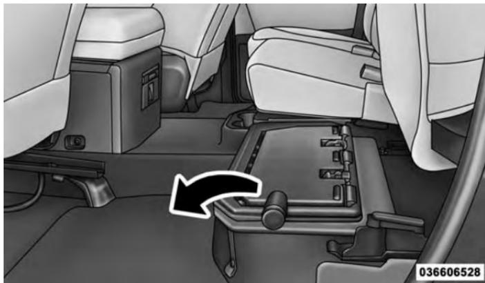
**Unfolding The Load Floor**
