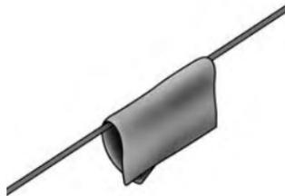
In certain situations you may decide to throw a heavy blanket or similar object over the wire rope. A heavy blanket can absorb energy should the wire rope break. Place it on the wire rope midway between the winch and the anchor point. Do this before the wire rope is put under tension. Do not approach
