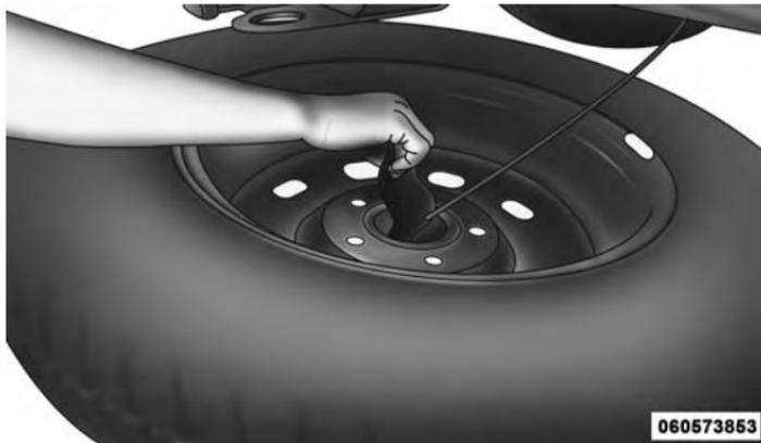
Reinstalling The Retainer
