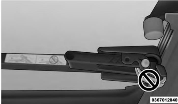
Improper Clamp Wire Released Position
