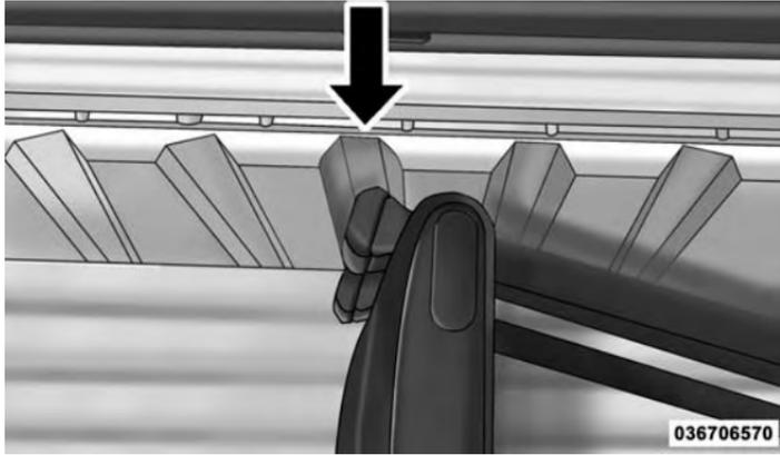
Aligning Gate To Slots
