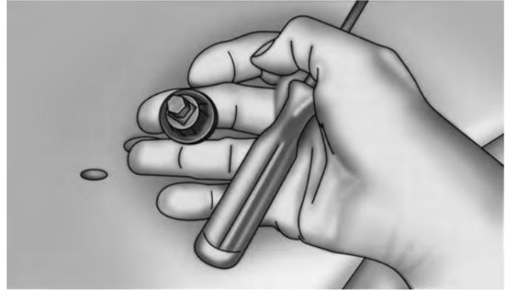
Removing The Bulb From The Bulb Socket
