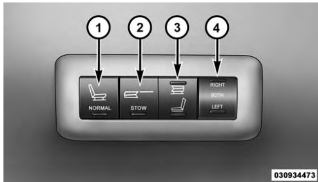
Rear Panel Power Switch Bank
