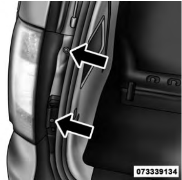
Tail Lamp Mounting Screws
