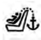
In addition, there are tether strap anchorages behind each rear seating position located in the panel between the rear seatback and the rear window. They are found under a plastic cover with the tether anchorage symbol on it.
