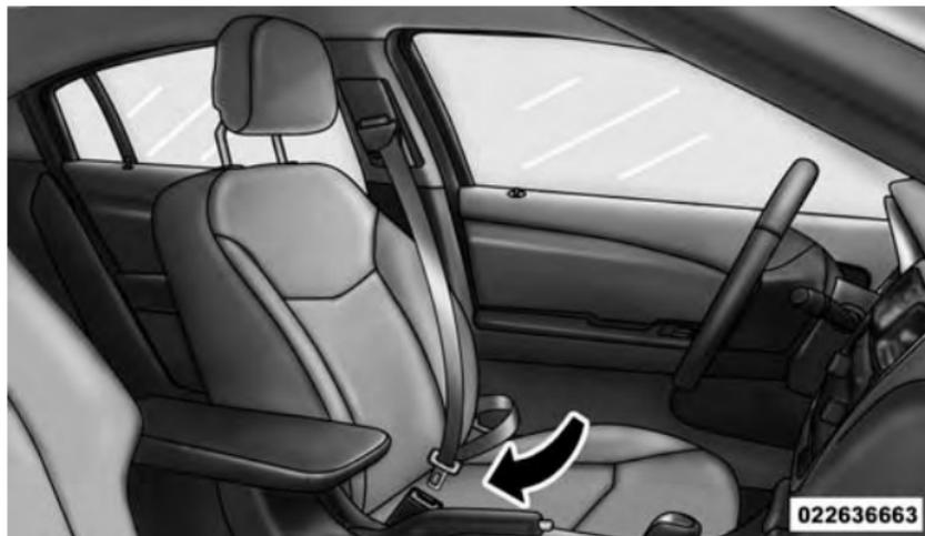
Inserting Latch Plate Into Buckle
