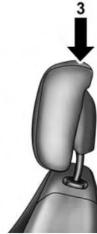
3 — Final Downward Movement To Engage Locking Mechanism
