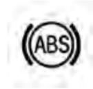
This light monitors the Anti-Lock Brake System (ABS). The light will turn on when the ignition switch is placed in the ON/RUN position and may stay on for as long as four seconds.
