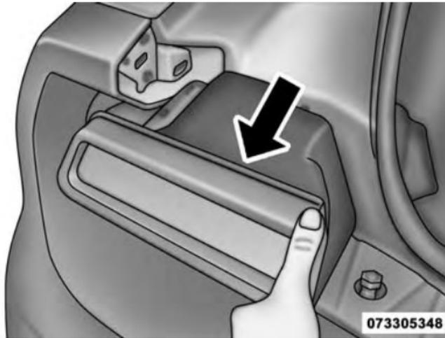
Removing Tail Lamp Assembly
