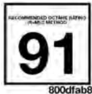
The 6.4L engine is designed to meet all emissions regulations and provide excellent fuel economy and performance when using high-quality premium unleaded gasoline with an octane rating of 91 or
