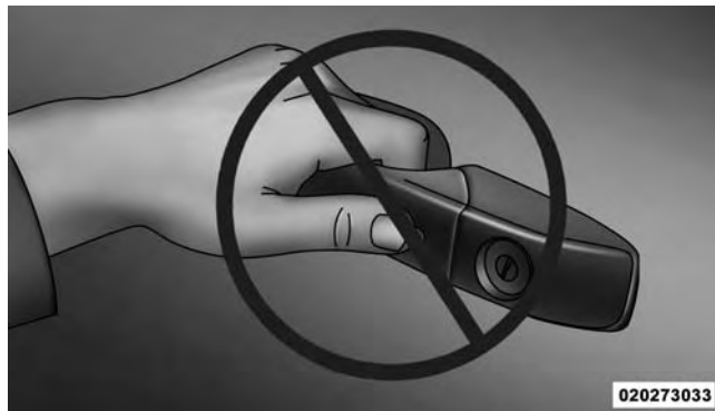
Do NOT Grab The Handle When Locking
