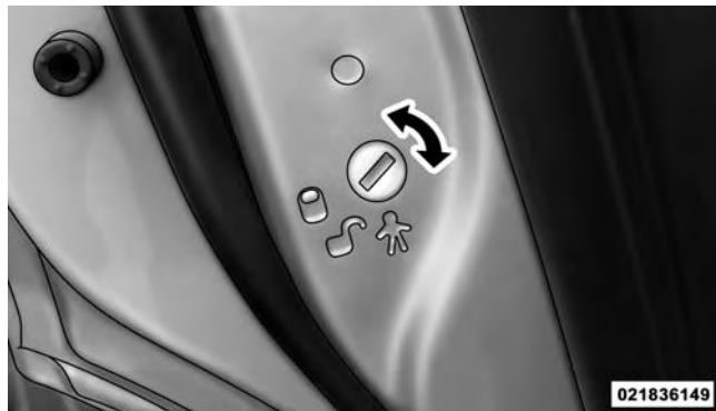
Child-Protection Door Lock Function
