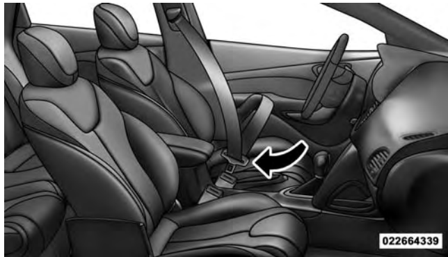
Inserting Latch Plate Into Buckle
