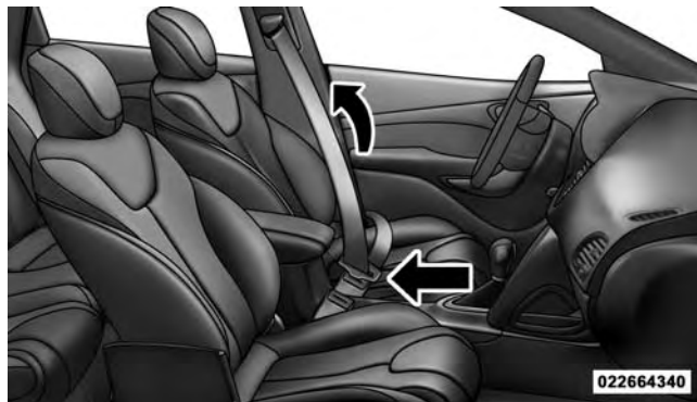
Removing Slack From Belt
