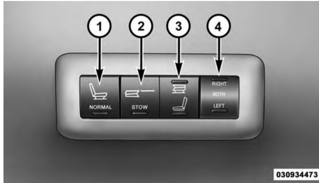
Rear Panel Power Switch Bank
