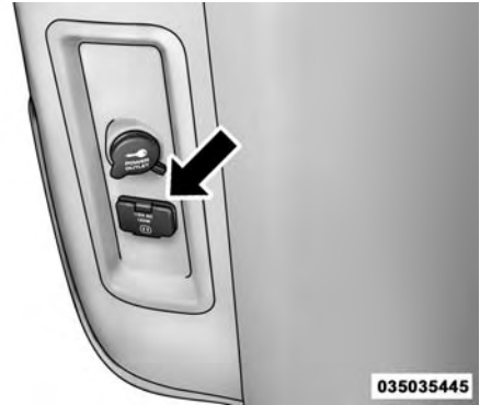
Power Inverter Outlet
