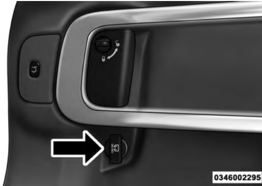
Rear Power Outlet
