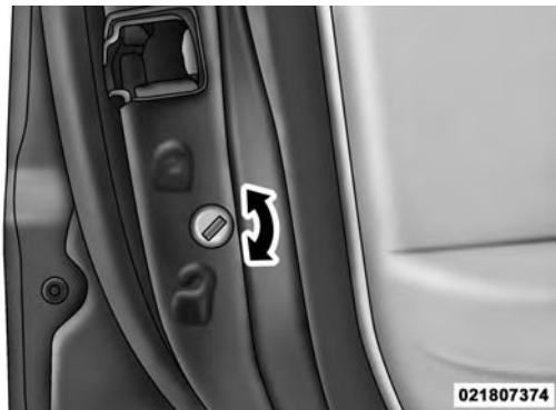
Child-Protection Door Lock Function
