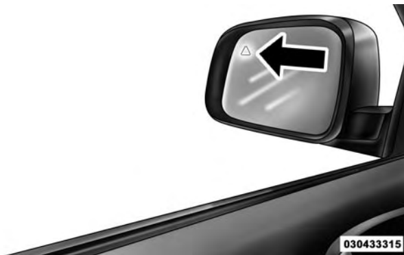
Warning Light Location
