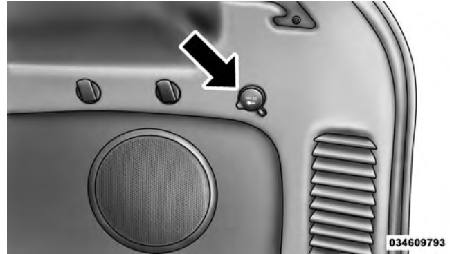
Rear Power Outlet
