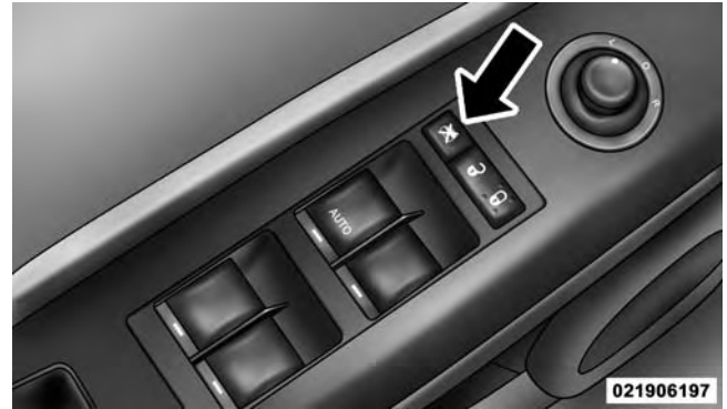
Window Lockout Switch
