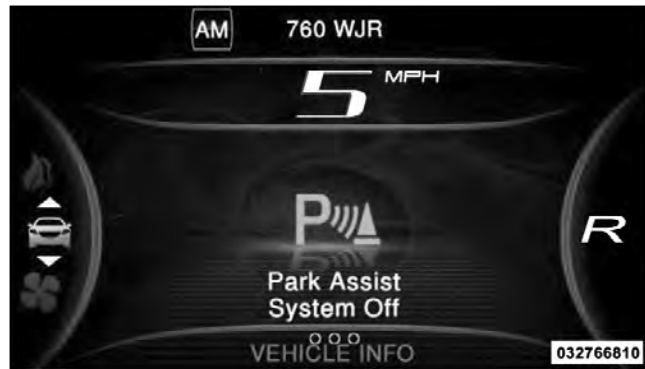
Park Assist System Off
