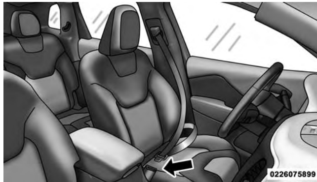
Inserting Latch Plate Into Buckle
