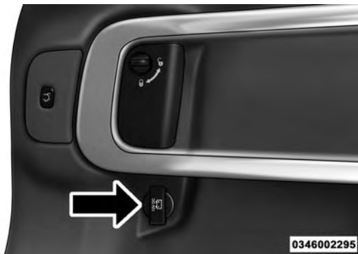
Rear Power Outlet
