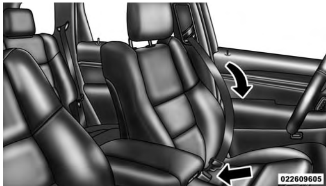
Pulling Out The Latch Plate
