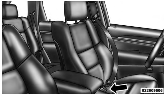
Inserting Latch Plate Into Buckle
