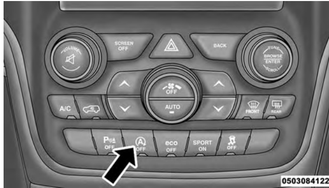
STOP/START Off Switch
