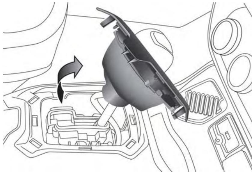
**Removing Gear Selector Bezel**
