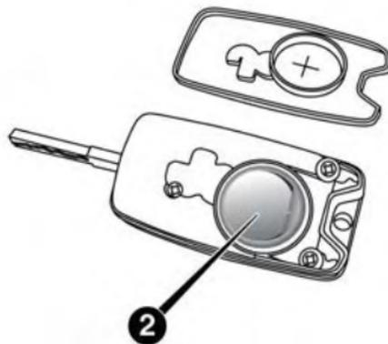
2 — Integrated Key Battery Removal
