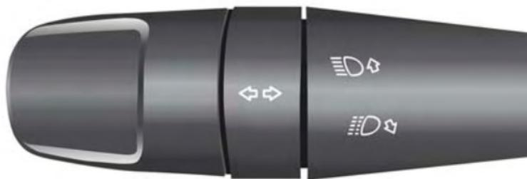
High Beam And Turn Signal Controls
