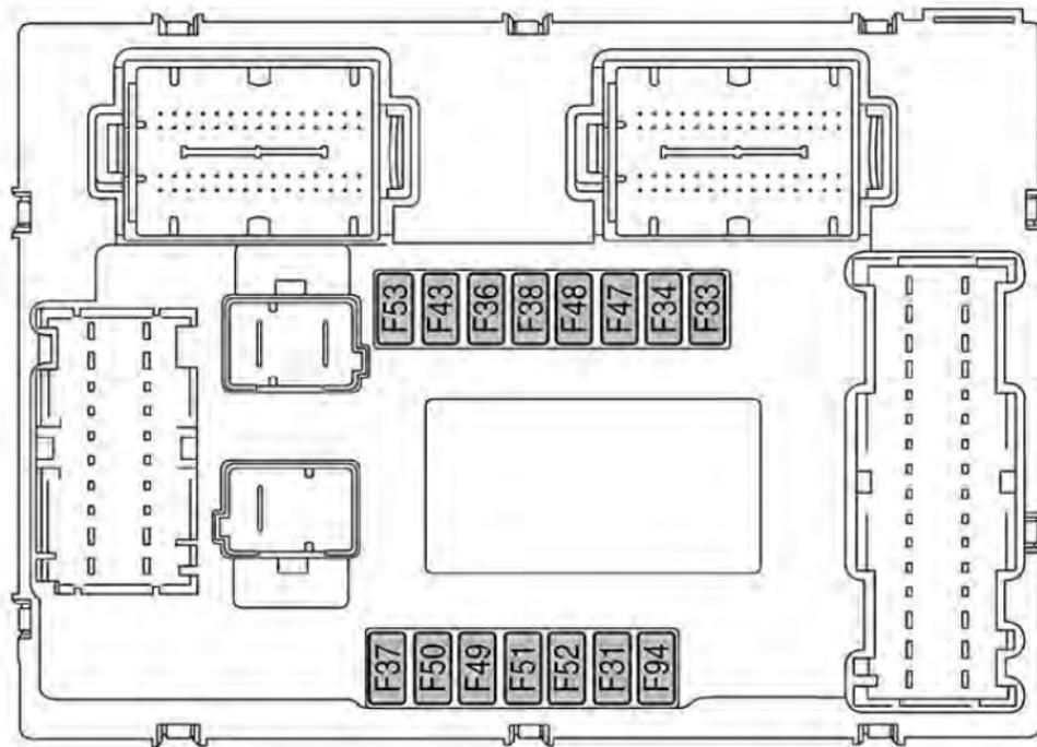
Body Controller Fuse Cavities
