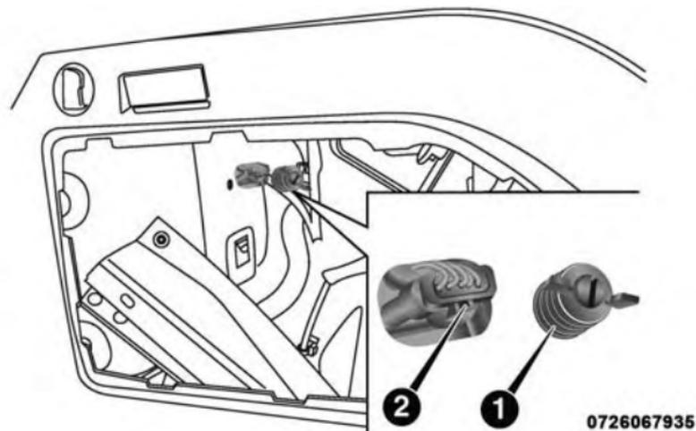
Rear Lamp Fastener and Electrical Connector
