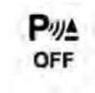
When the Rear ParkSense switch is pushed to disable the system, the instrument cluster will display the “PARKSENSE DISABLED” message
