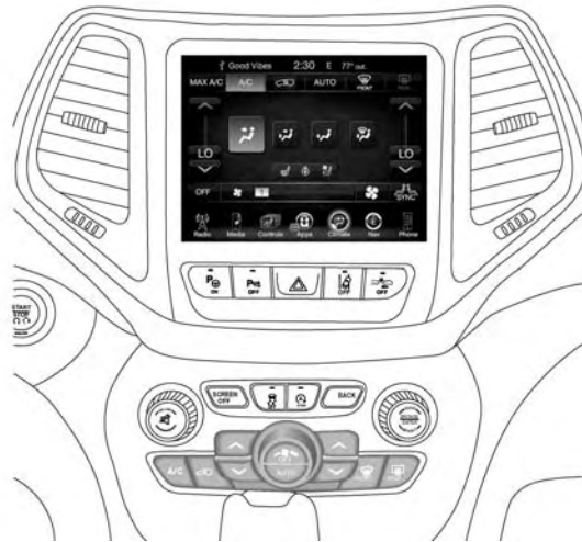
8.4/8.4 NAV With Automatic Temperature Controls
