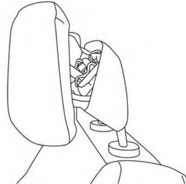
Active Head Restraint (AHR) Triggered
