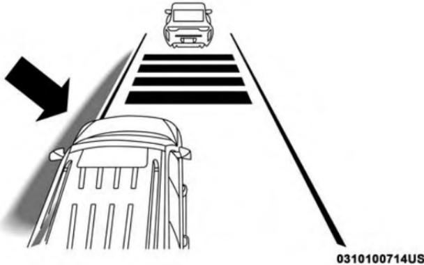
Lane Approached (Flashing Yellow Thick Line, Solid Yellow Thin Line/Flashing Yellow Telltale
