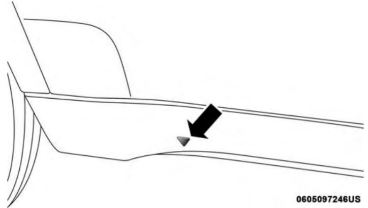
Lift Point Symbol On Sill Molding
