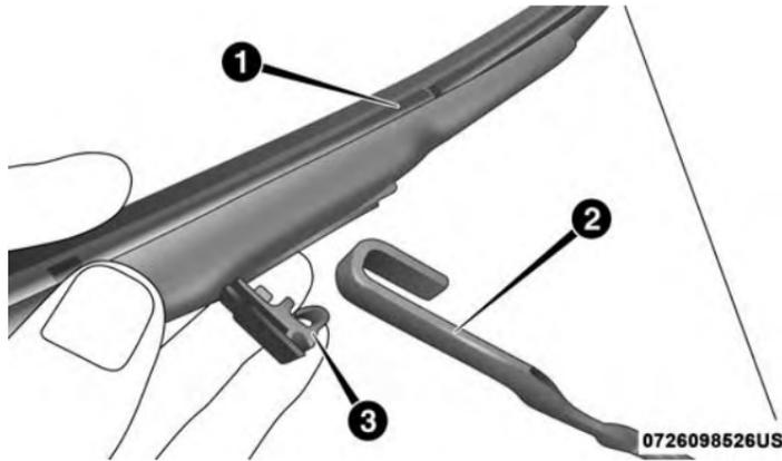
Wiper Blade Removed From Wiper Arm
