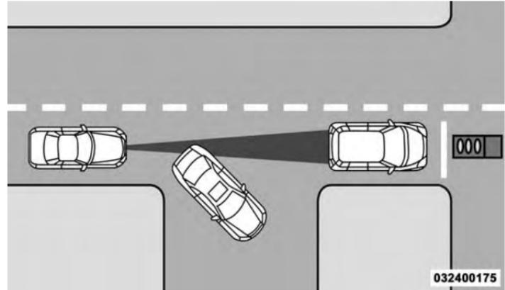
Stationary Object And Stationary Vehicle Example
