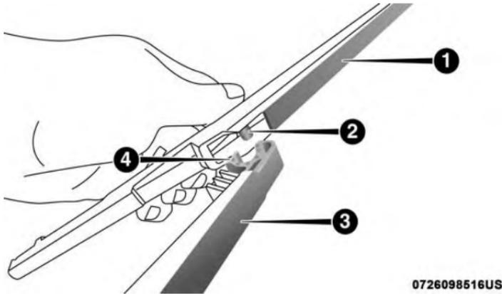
Wiper Blade Removed From Wiper Arm
