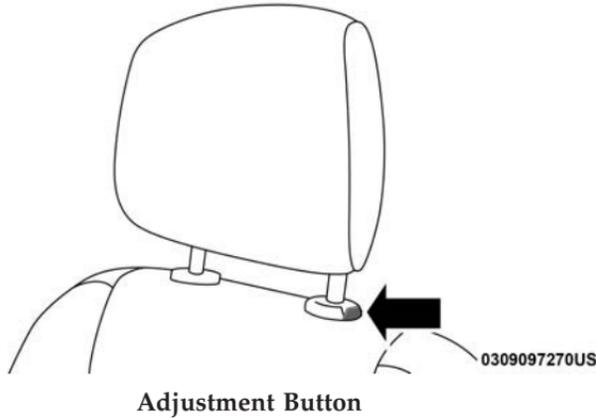
For comfort, the Active Head Restraints can be tilted forward and rearward. To tilt the head restraint closer to the back of your head, pull forward on the bottom of the head restraint. Push rearward on the bottom of the head restraint to move the head restraint away from your head.
