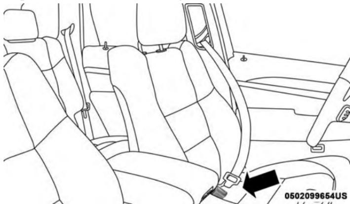
**Inserting Latch Plate Into Buckle**
