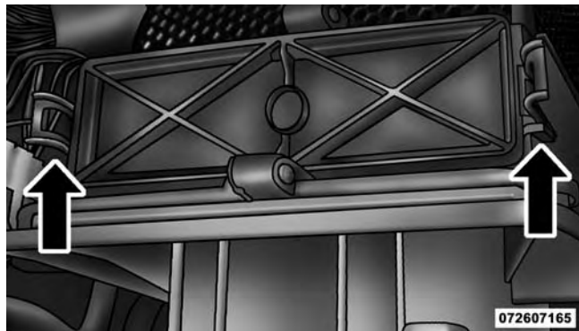
A/C Air Filter Replacement
