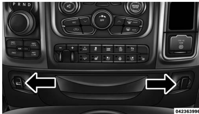
Power Outlets — Center Stack
