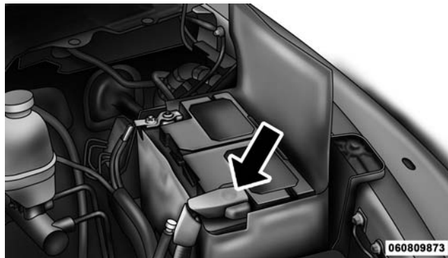
Positive Battery Post
