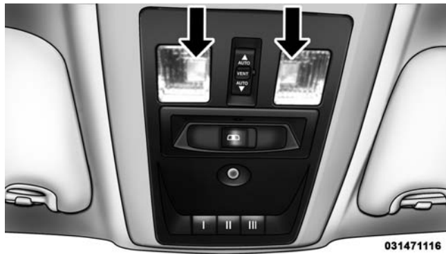
Front Courtesy/Reading Lights
