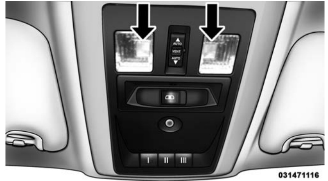
Front Courtesy/Reading Lights
