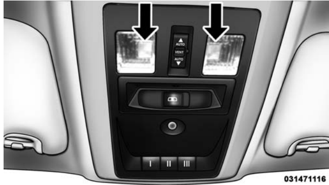
Front Courtesy/Reading Lights
