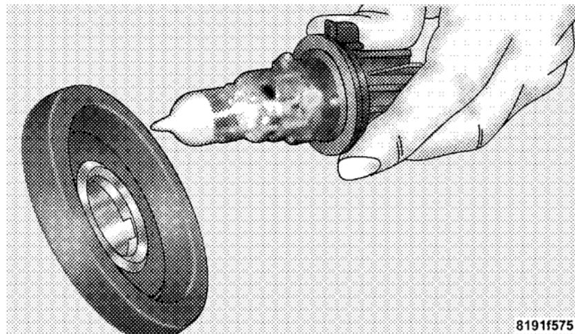
5. If the bulb comes in contact with any oily surface, clean the bulb with rubbing alcohol.
