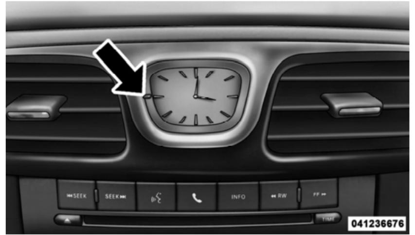
To set the analog clock, located at the top center of the instrument panel, press and hold the button in until the setting is correct. The clock will adjust slowly at first and then quicker the longer the button is held.
