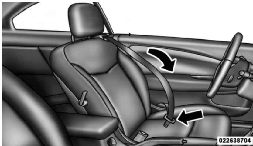
Inserting Latch Plate Into Buckle
