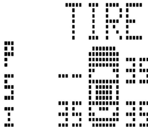
If the ignition key is cycled, this sequence will repeat, providing the system fault still exists. If the system fault no longer exists, the "Tire Pressure Monitoring Telltale Light" will no longer flash, and the "CHECK TPM SYSTEM" message will no longer display, and a pressure value will display in place of the dashes. A system fault can occur due to any of the following:
