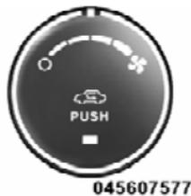
Rotate this control to regulate the amount of air forced through the ventilation system in any mode. The blower speed increases as you move the control to the right from the "O" (OFF) position. There are four blower speeds.
