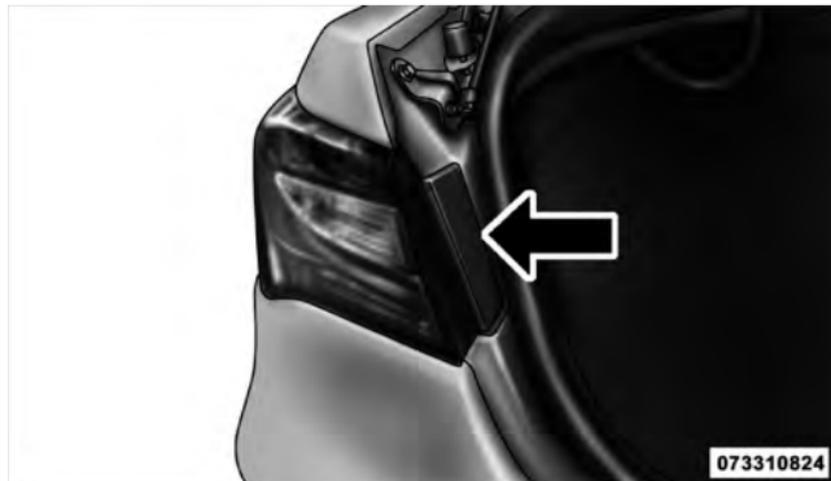
4. Twist and remove socket from lamp.
