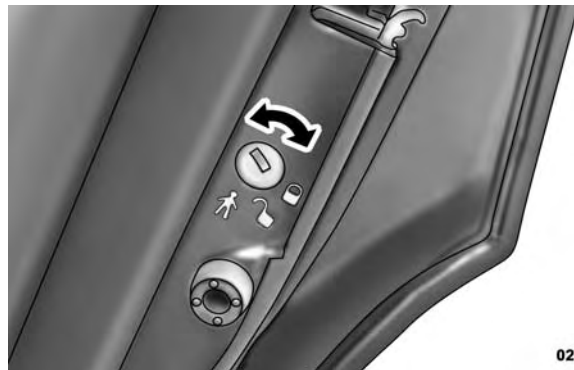
Child-Protection Door Lock Function
